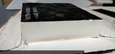
Shuttle Tile cross-section with HRSI coating removed
